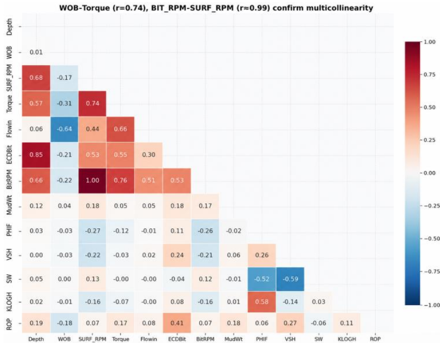
Figure 6: Pearson correlation matrix showing strong collinearity between BIT_RPM and SURF_RPM ( r \approx 0.99 )
